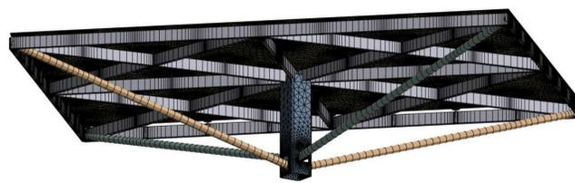
Fig. 3 Finite element model of heliostat frame
