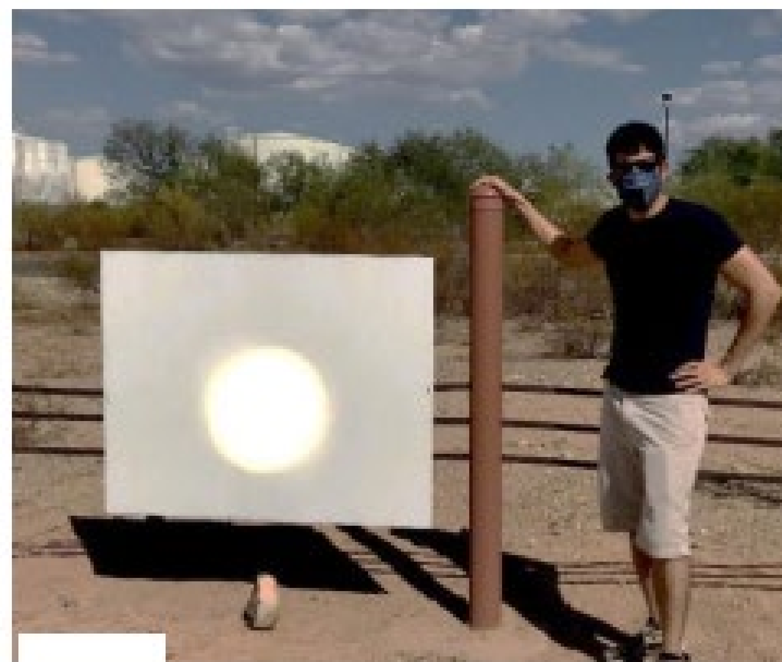
Solar disc image formed late in the day (angle of incidence 60°) by a single 1.6 m 2 twisting mirror heliostat at 40 m distance. Similar quality solar images are achieved throughout the day.
