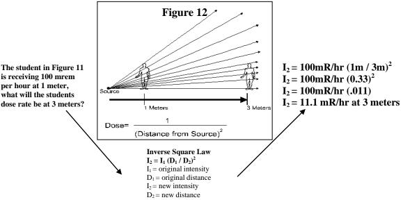
Both irradiation facilities are designed to have their operators outside of the shielded irradiator room while the source is exposed in order to take advantage of distance.
