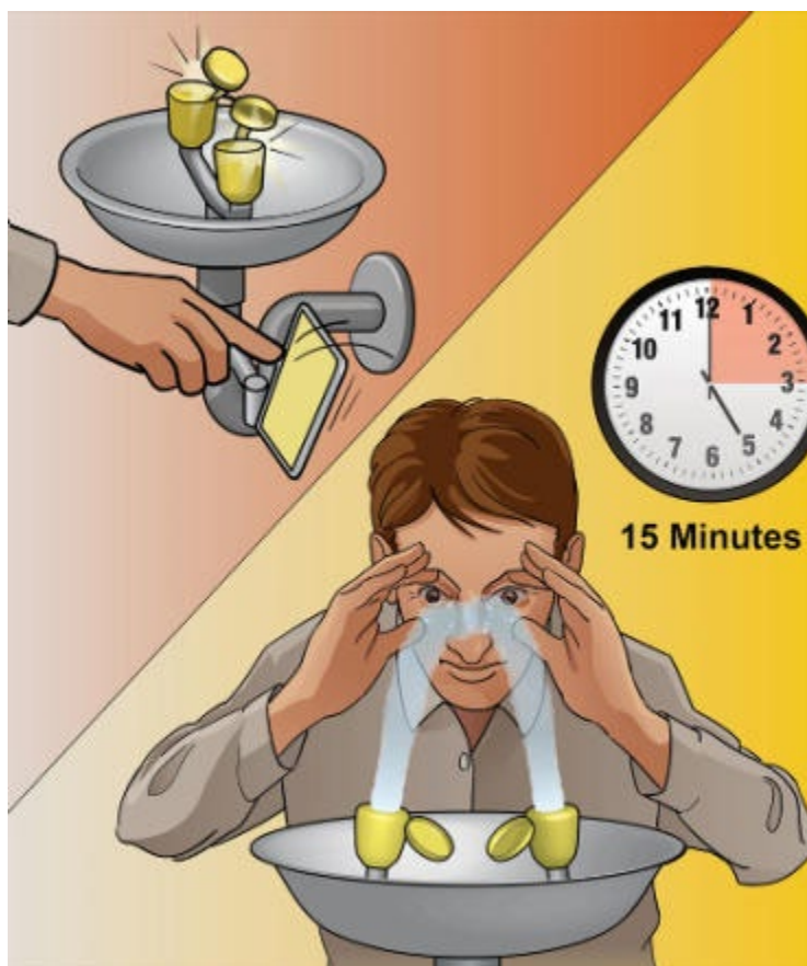
Figure 9. Always rinse eyes for at least 15 minutes when using an emergency eyewash station.
