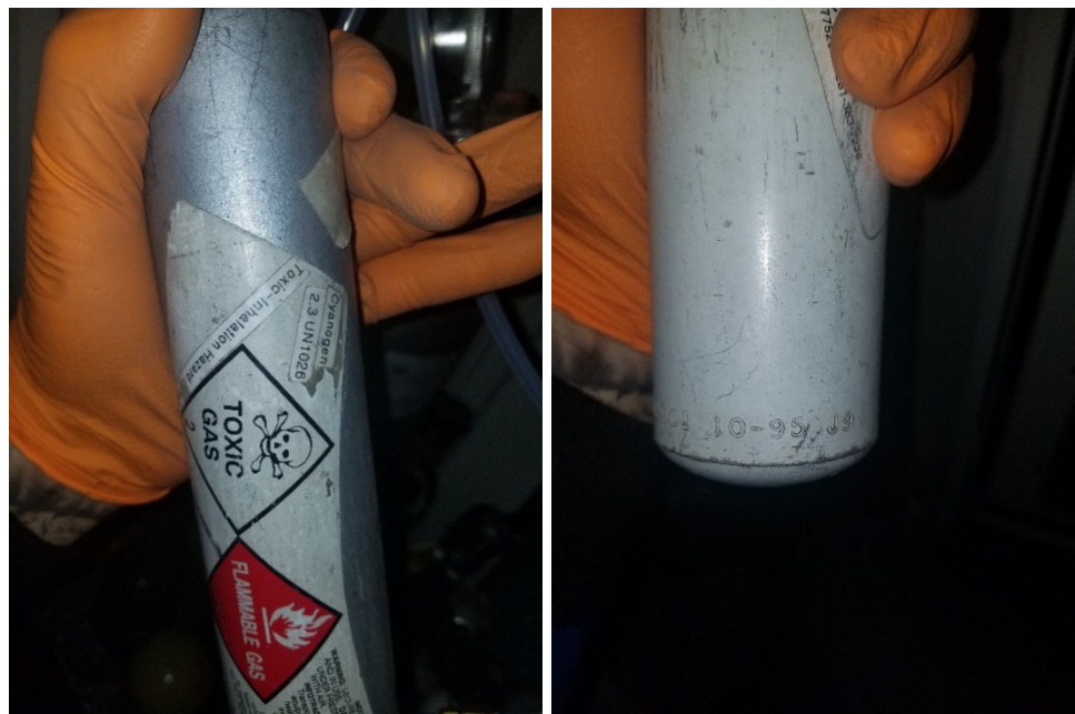
Figure 16. Gas lecture bottles are small and easily held in the hand. This cylinder of cyanogen gas bottled in October 1995 was submitted as hazardous waste in June 2023 – almost 28 years after it had been initially filled!
