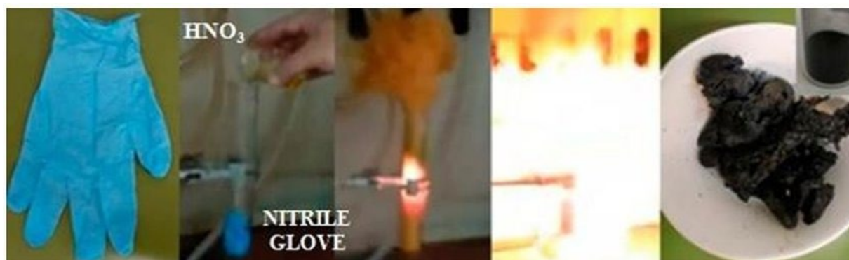
Figure 22. Fuming nitric acid, a very powerful oxidizer, can react with nitrile gloves to result in a combustion reaction.
